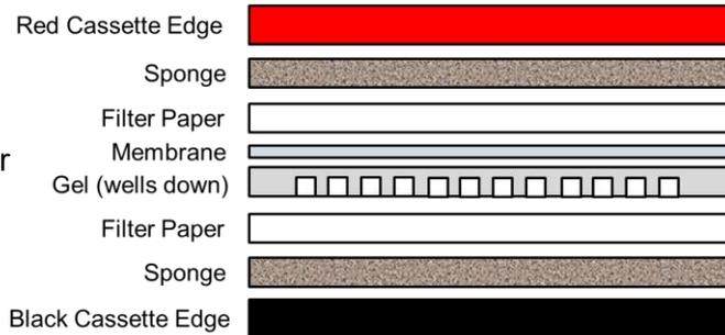
10. Carefully close and clamp the cassette. The final assembly is pictured.
